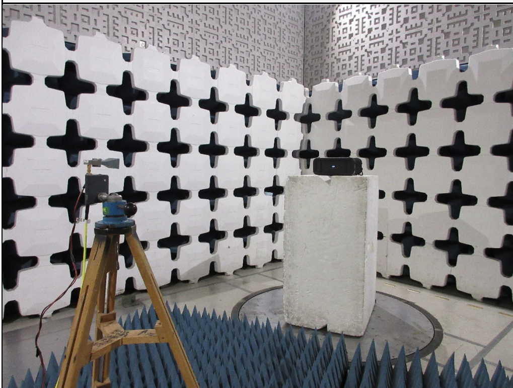
Test Setup for Spurious Radiated Emissions, Above 18GHz – Antenna Polarization Vertical
