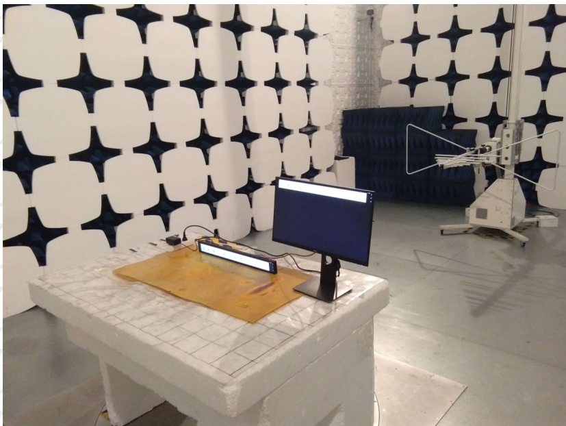
Photograph of test setup for Radiated Emission below 1 G
