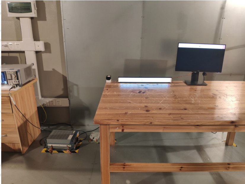
Photograph of test setup for Conducted Emission
