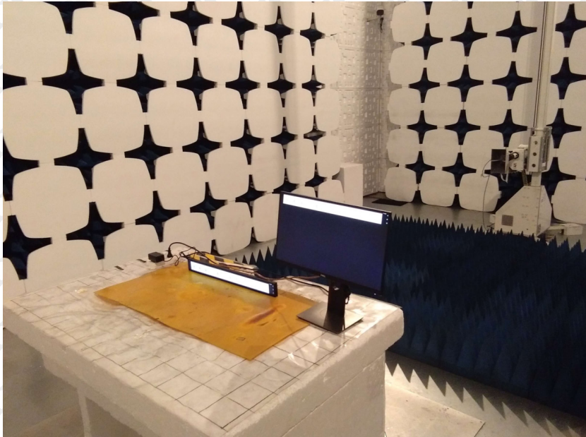
Photograph of test setup for Radiated Emission above 1 G
