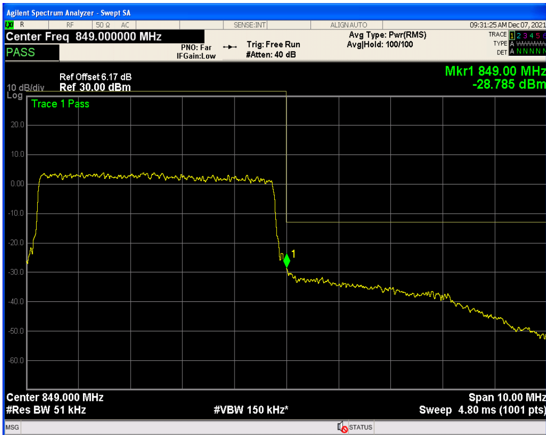
Band5 QAM16 BW=5MHz Channel=20625 RB Size=1 Position=#Max
