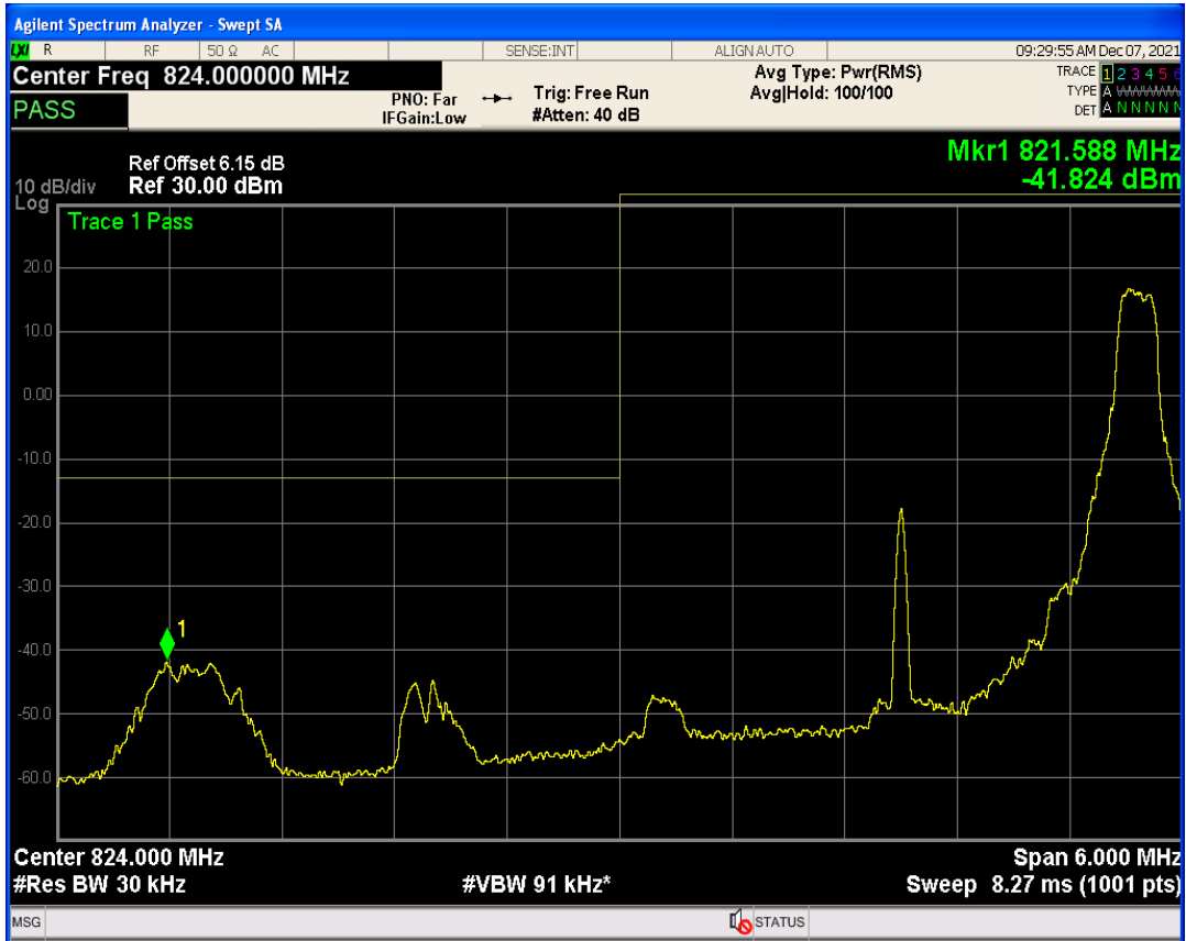
Band5 QPSK BW=3MHz Channel=20415 RB Size=15 Position=#0
