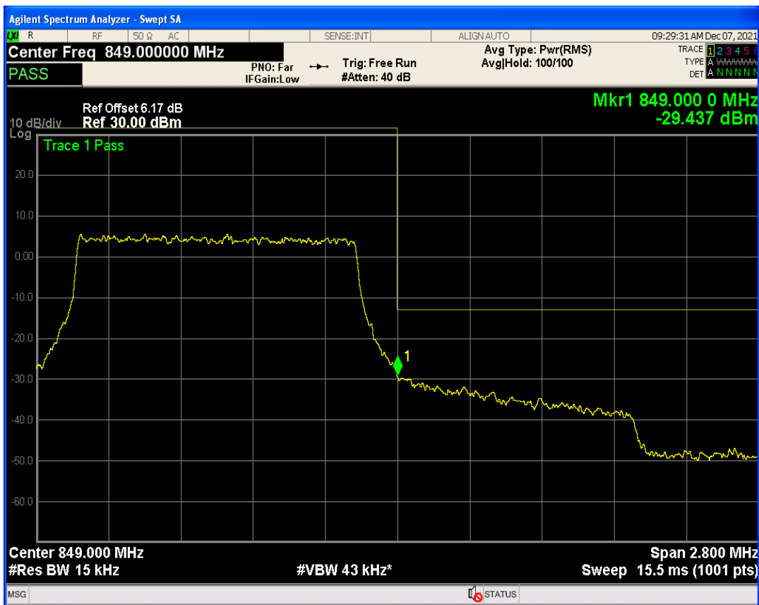
Band5 QAM16 BW=1.4MHz Channel=20643 RB Size=1 Position=#0
