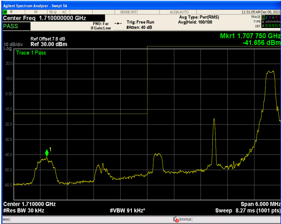
Band66 QPSK BW=3MHz Channel=132657 RB Size=1 Position=#Max
