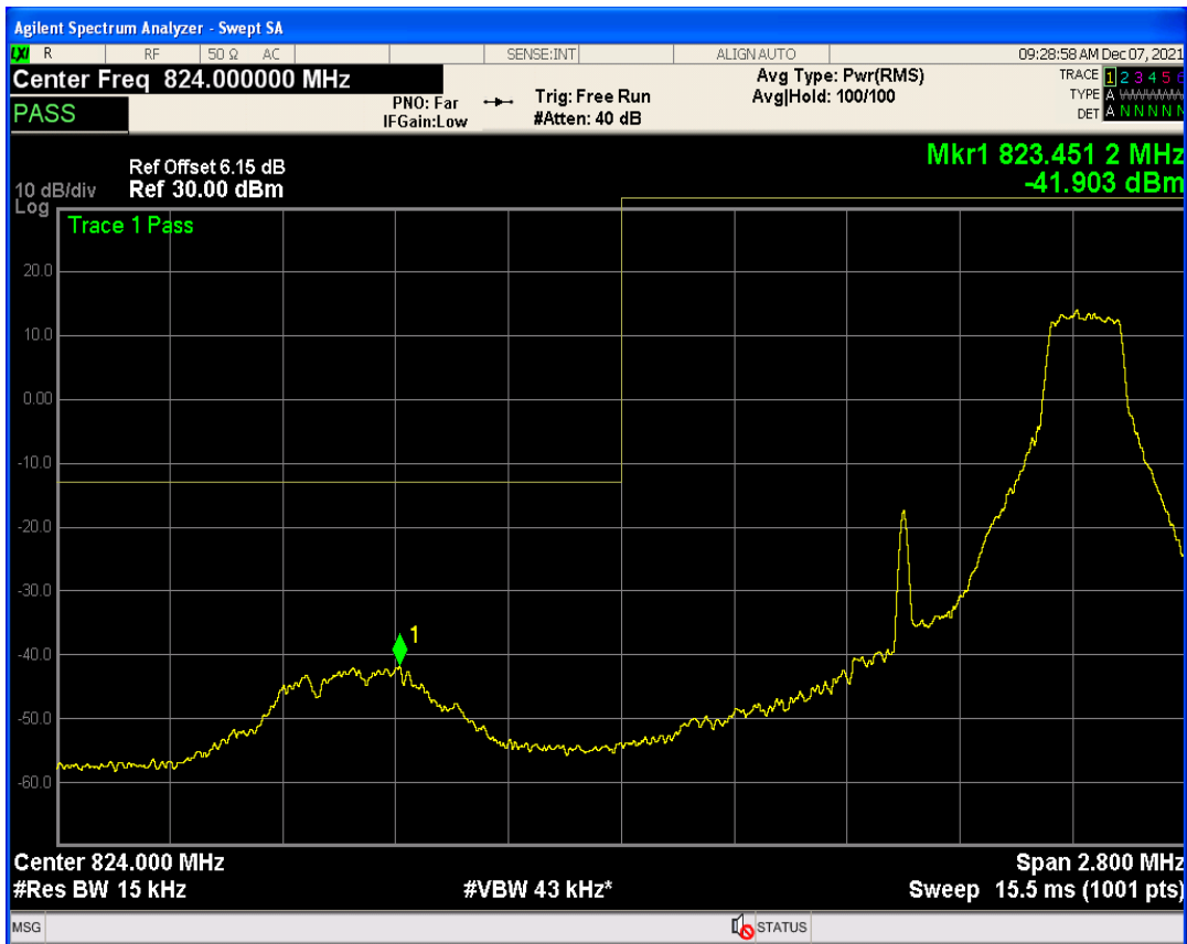
Band5 QAM16 BW=1.4MHz Channel=20407 RB Size=1 Position=#0
