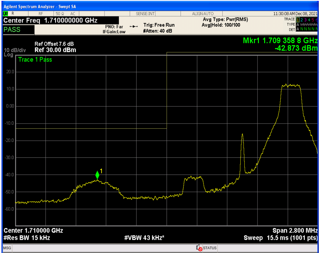
Band66 QPSK BW=1.4MHz Channel=132665 RB Size=1 Position=#0
