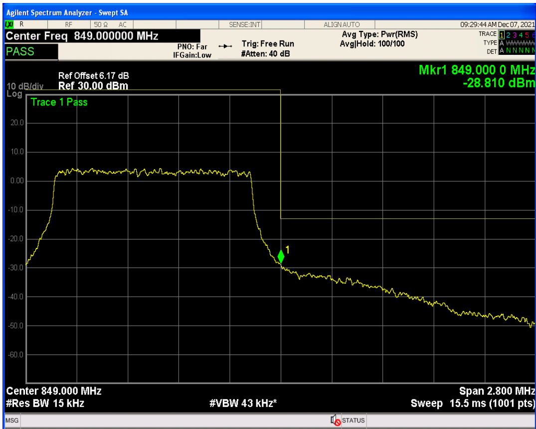
Band5 QPSK BW=3MHz Channel=20415 RB Size=1 Position=#0
