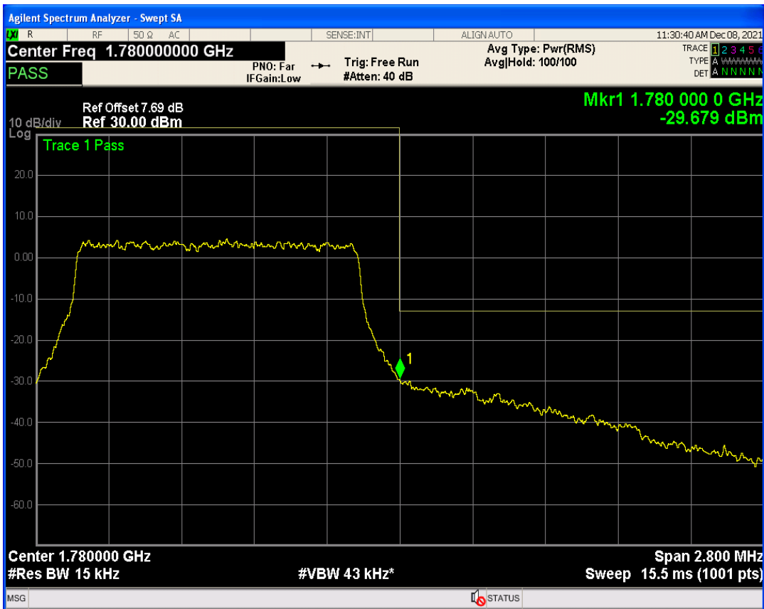
Band66 QAM16 BW=1.4MHz Channel=132665 RB Size=1 Position=#Max
