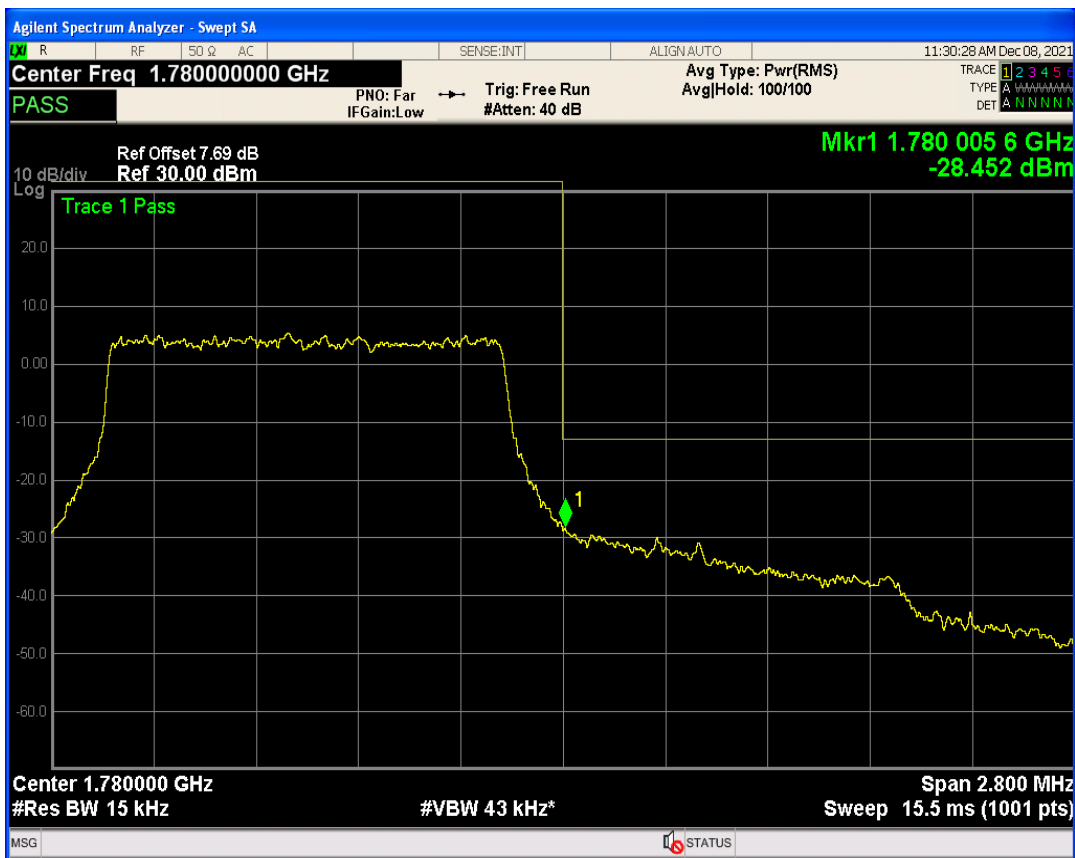
Band66 QAM16 BW=1.4MHz Channel=132665 RB Size=1 Position=#0
