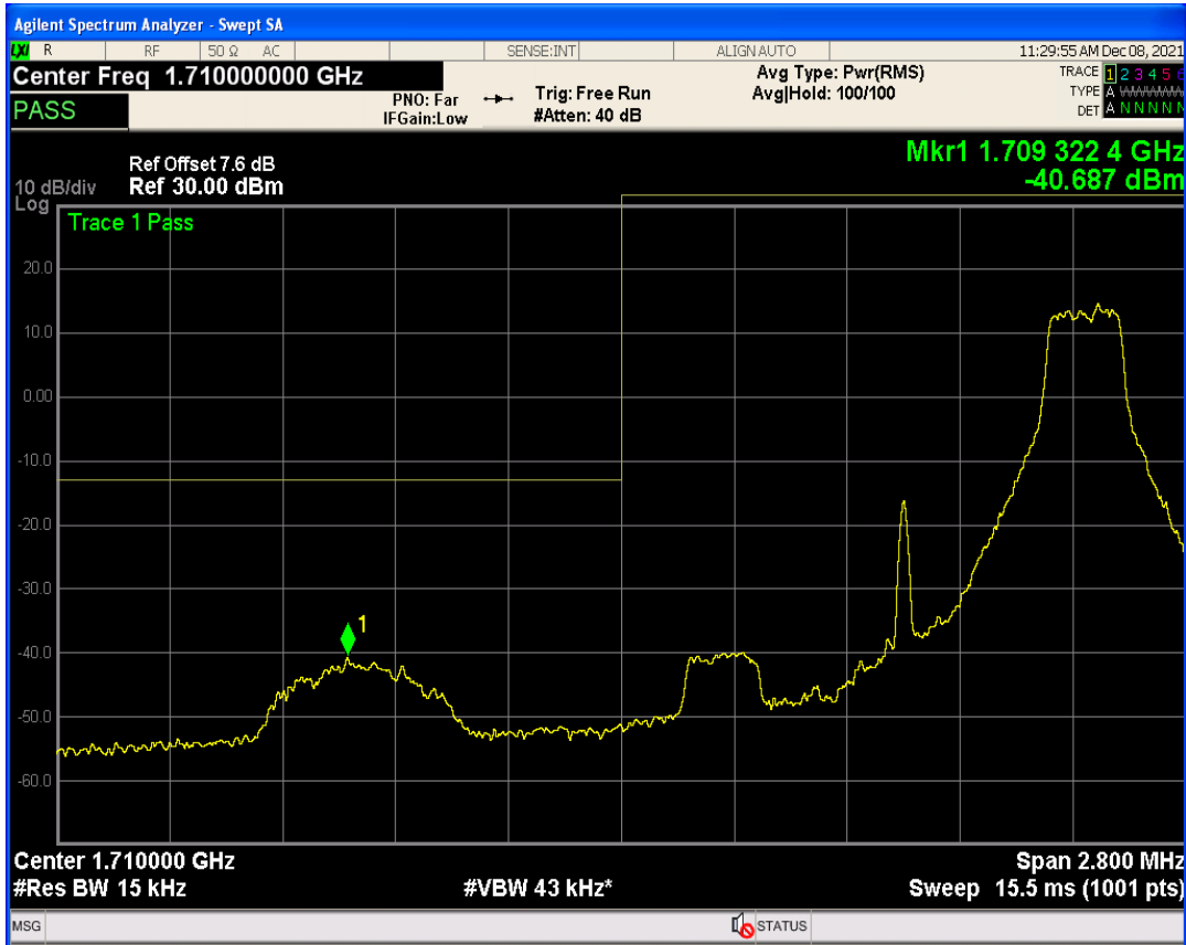
Band66 QAM16 BW=1.4MHz Channel=131979 RB Size=1 Position=#0
