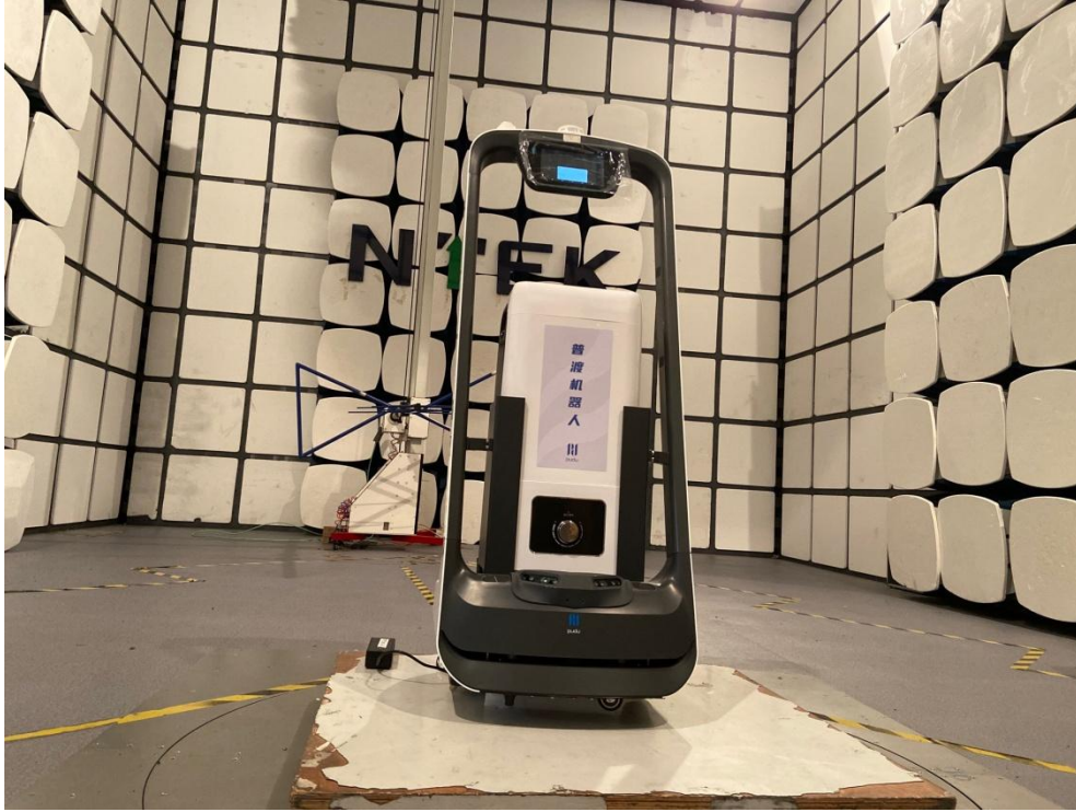
Radiated Measurement Photos(30MHz~1GHz )
