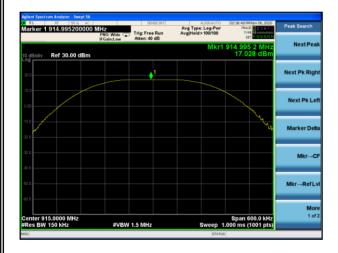
Peak output Power plot on channel 60
