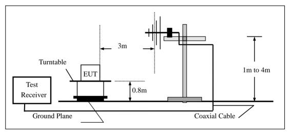
(c) For radiated emissions above 1000MHz
