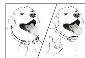
Note: It is sometimes necessary to trim the hair around the Contact Points to make sure that the contact electrodes delivers effective static.
