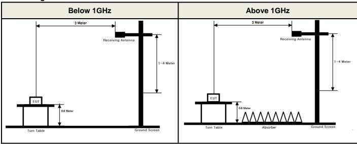
These measurements were performed at 3 m test site. The equipment under test is placed on a non-conductive table 1.5 meters above a turntable which is flush with the ground plane and 3 meters from the receive antenna. For measurements above 1GHz absorbers are placed on the floor between the turn table and the antenna mast in such a way so as to maximize the reduction of reflections. For measurements below 1 GHz, the absorbers are removed.
