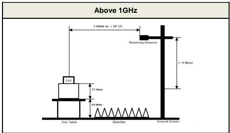
These measurements were performed at 3 m test site. The equipment under test is placed on a non-conductive table 1.5-meters above a turntable which is flush with the ground plane and 3 meters from the receive antenna. For measurements above 1GHz absorbers are placed on the floor between the turn table and the antenna mast in such a way so as to maximize the reduction of reflections.
