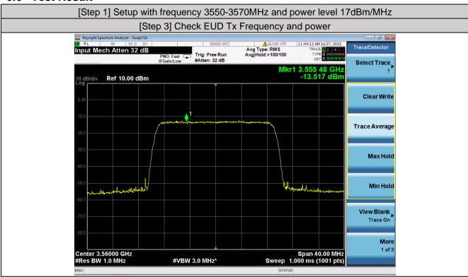
EIRP PSD=-13.517-6.1+15=-4.617dBm/MHz, attenuation of Cable and Splitter is 15dB, Antenna gain is - 6.1dBi.
