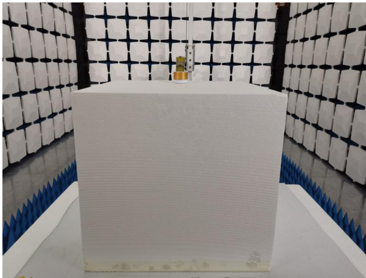
Above 1GHz for radiated emission test setup
