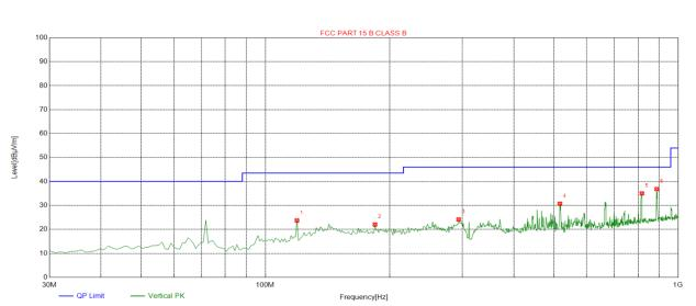
Suspected List Reading Freq. Factor Limit Margin Height Level Angle NO. Polarity [MHz] [dB]  $[dB\mu V/m]$  $[dB\mu V/m]$  $[dB\mu V/m]$ [dB] [cm] [°] 119.3293 40.70 23.71 43.50 -16.99 19.79 100 307 1 Vertical 2 184.3844 -16.48 38.51 22.03 43.50 21.47 100 174 Vertical 294.1041 -12.80 24.15 46.00 21.85 171 Vertical 3 36.95 100 -7.80 15.27 517.4274 38.53 30.73 46.00 126 Vertical 4 100 -2.77 5 817.4575 37.81 35.04 46.00 10.96 100 104 Vertical 6 888.3383 -1.91 38.74 36.83 46.00 9.17 100 326 Vertical
