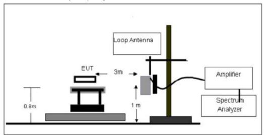
(B) Radiated Emission Test-Up Frequency 30MHz~1GHz
