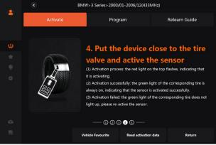
Figure 3-5 Sample Activation Operation Interface
