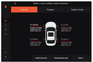
Figure 3-7 Sample Get Tire Pressure Data Interface
