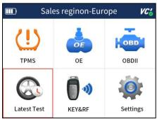
Scroll with the UP/DOWN arrow keys to choose one test record from the history diagnostic records and press the YES key to start.
