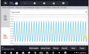
Figure 5-21 Sample PID Graph Screen
