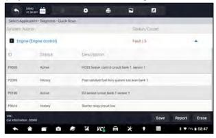
Figure 5-4 Sample Quick Scan Complete Screen
