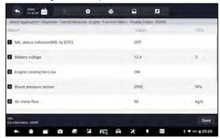
Figure 5-13 Sample Freeze Frame Screen
