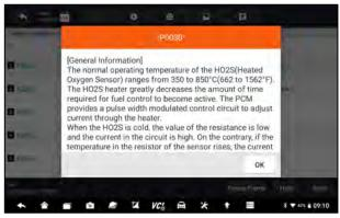
Figure 5-14 Sample DTC Help Screen
