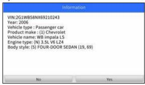
Figure 4-13 Sample Automatic VIN Reading Screen
