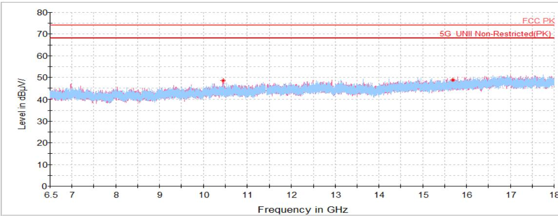
**802.11ac VHT20 UNII 1 ANT 0****Lowest Channel (5 180 MHz)**
