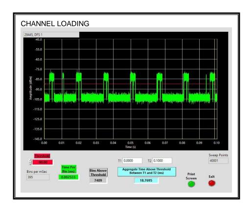
The level of traffic loading on the channel by the EUT is 18.77%
