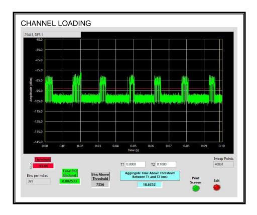
The level of traffic loading on the channel by the EUT is 18.63%
