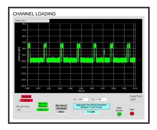
The level of traffic loading on the channel by the EUT is 17.39%
