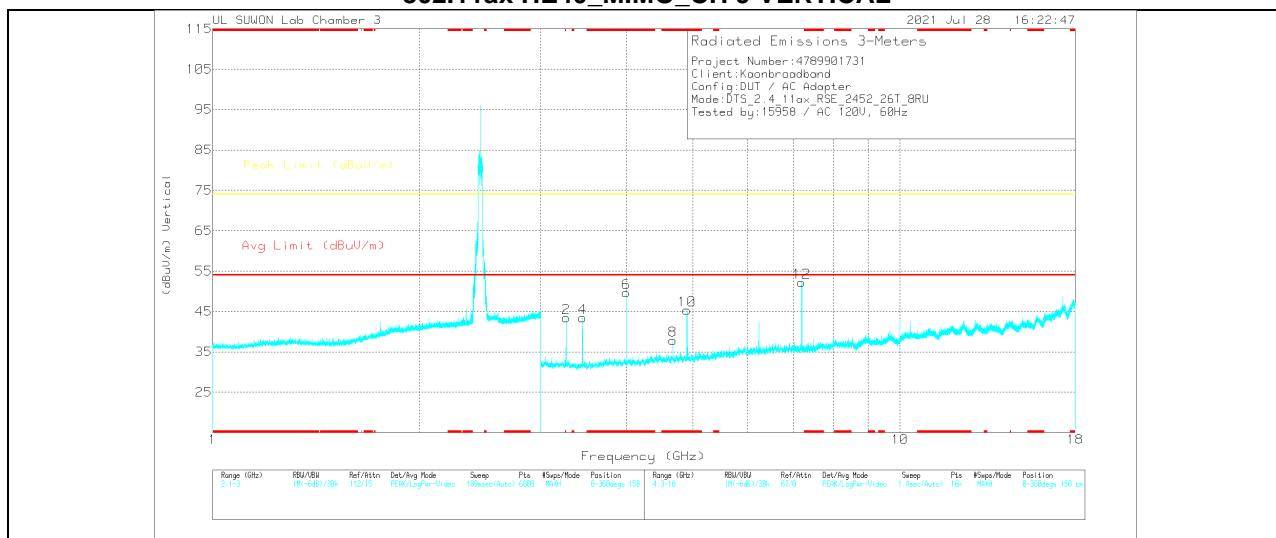
Note: Emission was scanned up to 26GHz; No emissions were detected above the noise floor which was at least 20dB below the specification limit.
