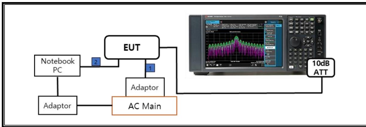
**SETUP DIAGRAM FOR TESTS (RADIATED TEST SETUP)**
