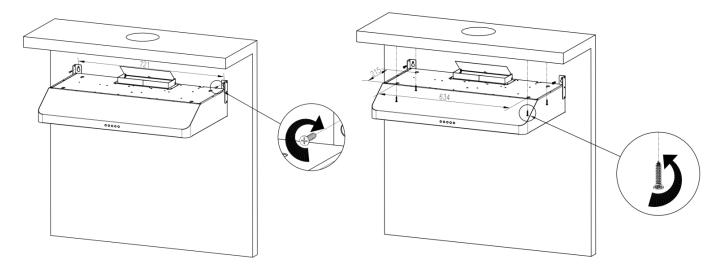
Wall mounted: 1.Drill two holes on the wall
