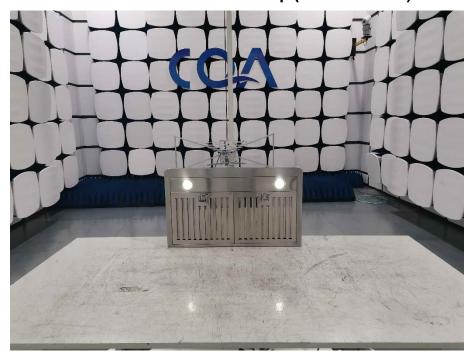
**Conducted Emissions Test Setup**
