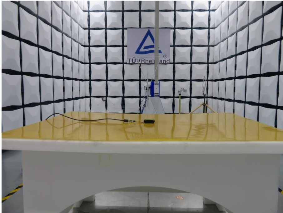
Photograph 1: Set-up for Radiated Spurious Emission, 30MHz - 1GHz
