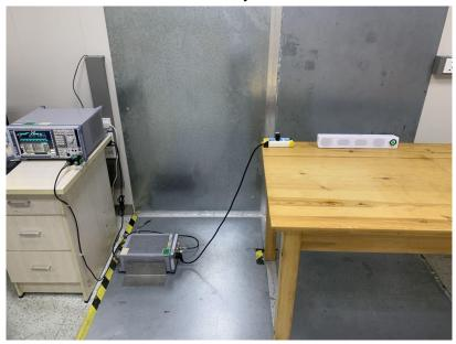
Radiated Spurious Emissions From 30MHz-1000MHz
