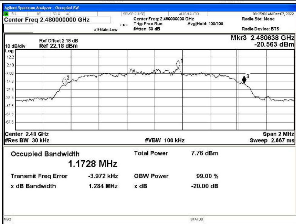
-20dB Bandwidth NVNT 2-DH5 2480MHz Ant1
