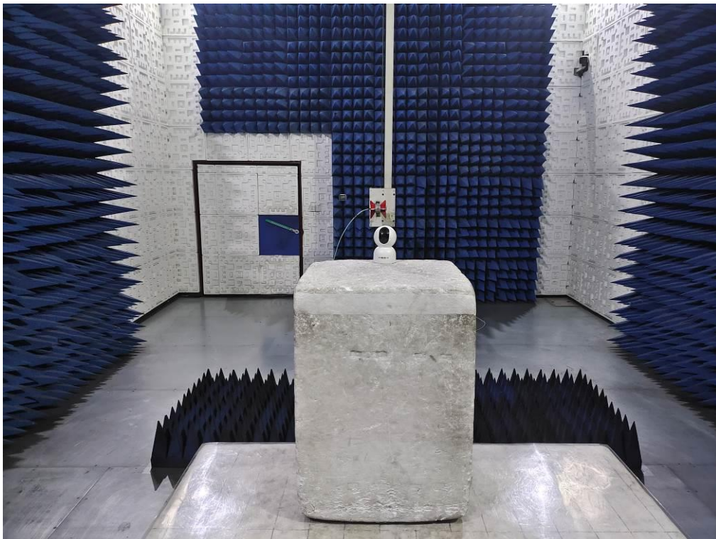
RADIATED EMISSION TEST SETUP ABOVE 1GHz
