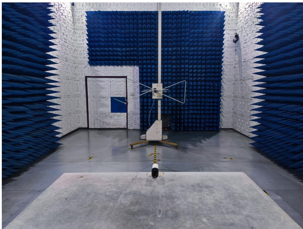
RADIATED EMISSION TEST SETUP ABOVE 1GHZ
