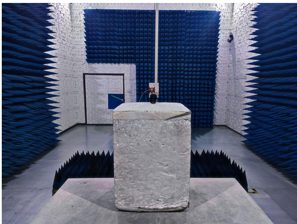
RADIATED EMISSION TEST SETUP ABOVE 1GHZ
