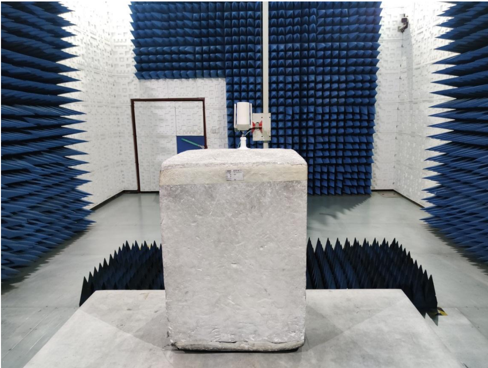
FCC RADIATED EMISSION TEST SETUP ABOVE 1GHZ
