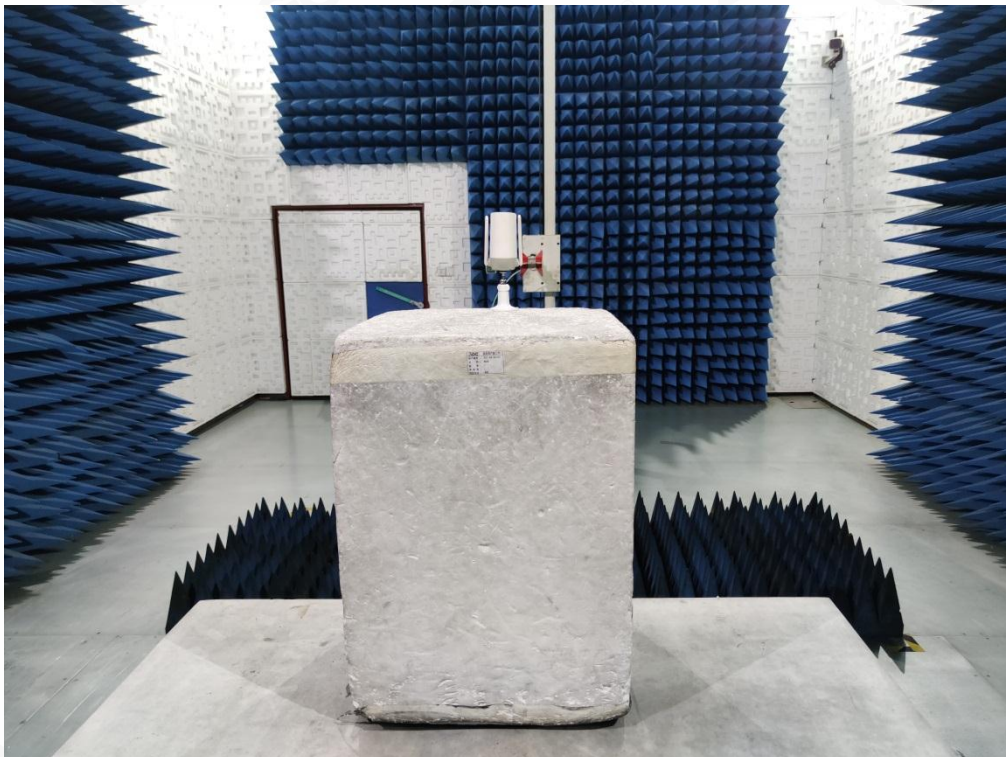
FCC RADIATED EMISSION TEST SETUP ABOVE 1GHZ
