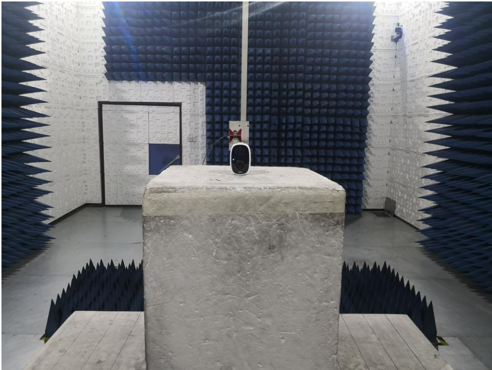
FCC RADIATED EMISSION TEST SETUP ABOVE 1GHZ
