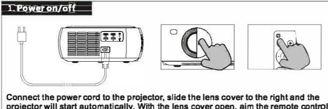
Connect the power cord to the projector, slide the lens cover to the right and the projector will start automatically. With the lens cover open, aim the remote control at the front/ rear infrared window of the fuselage, and press the "power key" to start the device.
