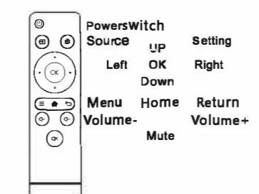
Note: The remote control must correspond to the infrared or screen of the fuselage to be effective.
