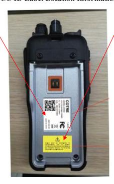
The label shown shall be permanently affixed at a conspicuous location on the device and be readily visible to the user at the time purchase (Labeling requirements per 2.925)
