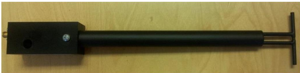
Figure 1 – MVG COMOSAR Validation Dipole
