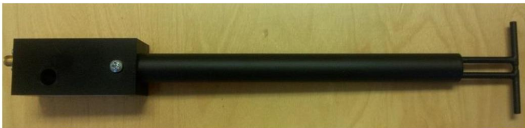
Figure 1 – MVG COMOSAR Validation Dipole
