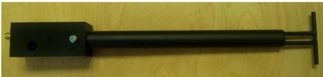
Figure 1 – MVG COMOSAR Validation Dipole
