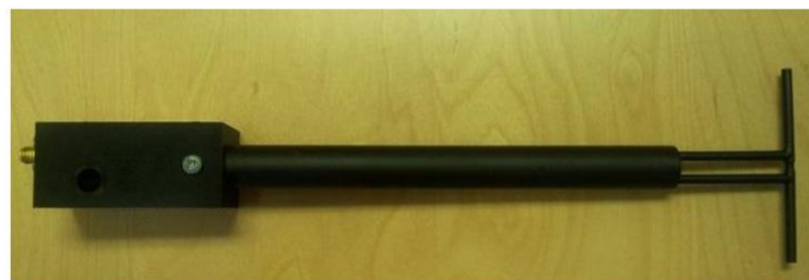
Figure 1 – MVG COMOSAR Validation Dipole
