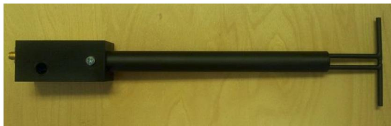
Figure 1 – MVG COMOSAR Validation Dipole
