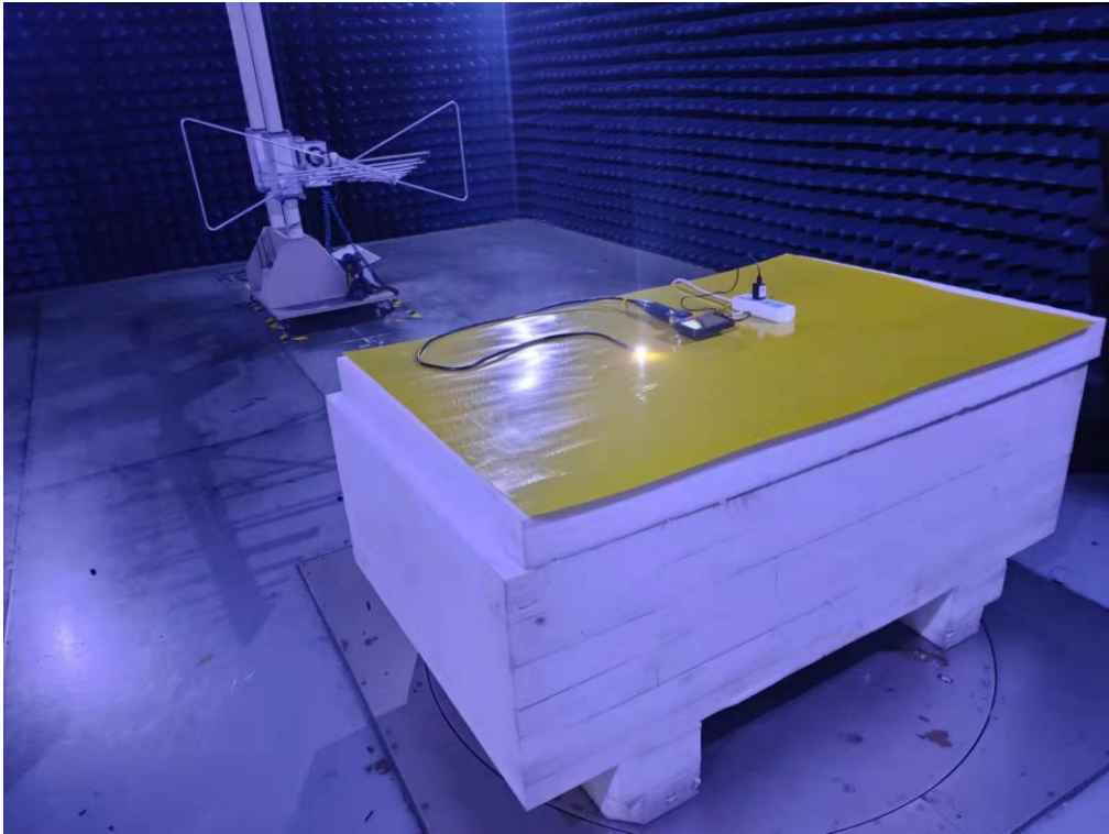
Photo of Radiated Emission Measurement (Below 1G)
