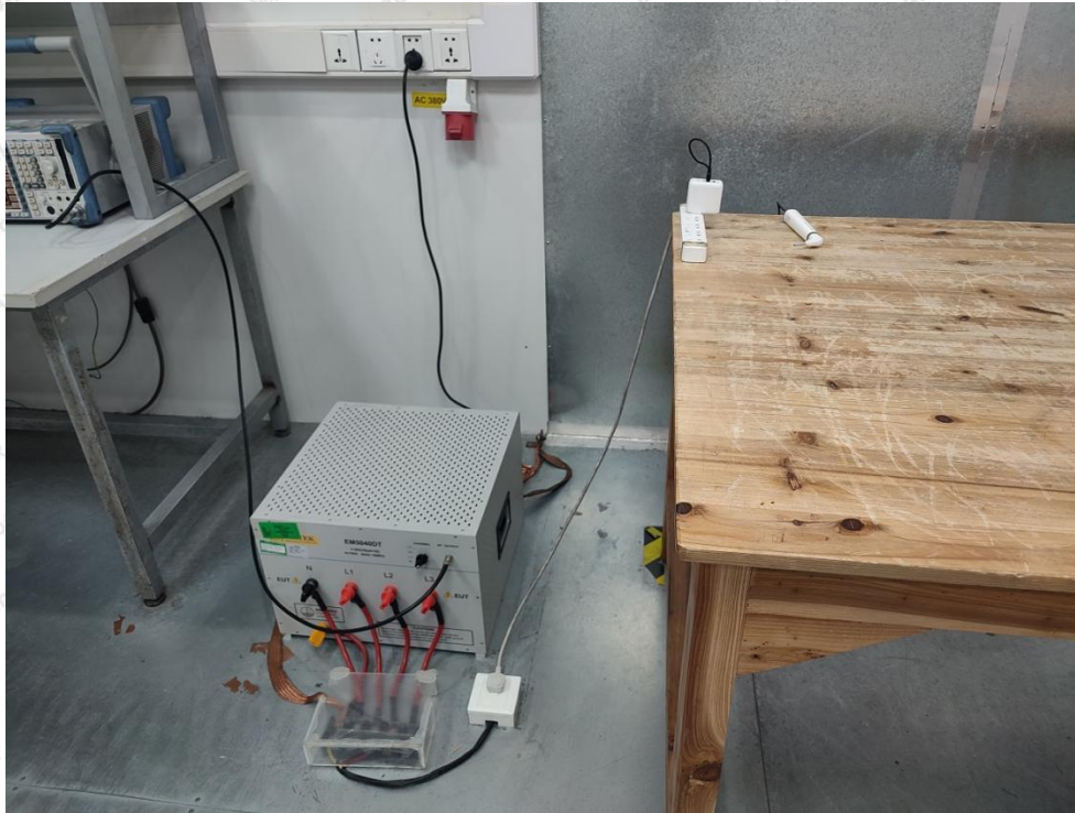
Photo of Power Line Conducted Emission Test
