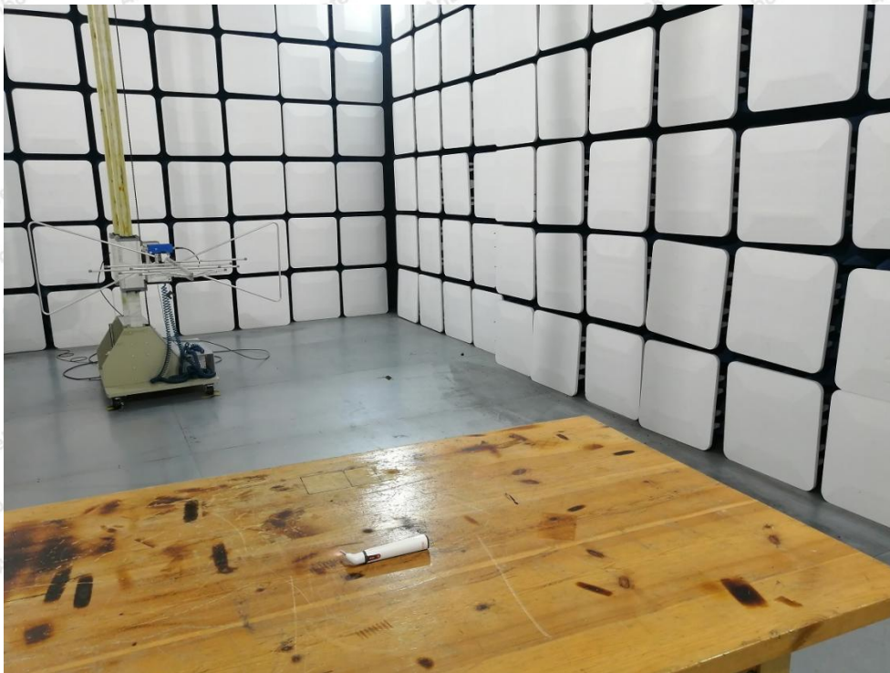
Photo of Radiation Emission Test
