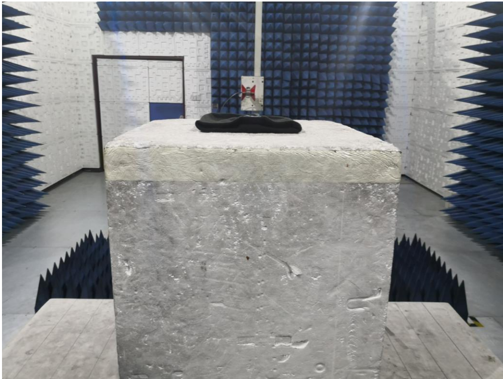
RADIATED EMISSION TEST SETUP ABOVE 1GHz
