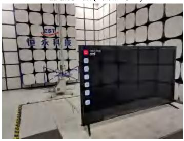
Radiated Test (Above 1GHz)
