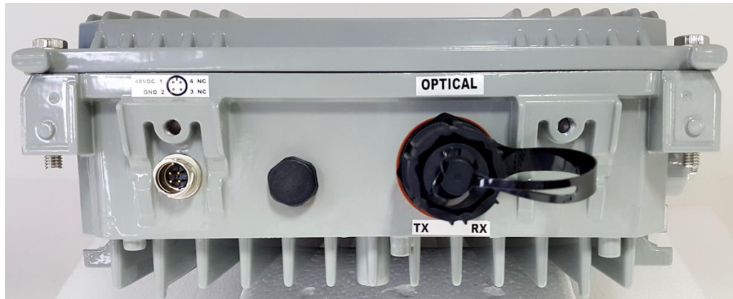
Figure 9. Equipment Unit DC and Fiber Optic Connections. The fiber connector is shown capped.
