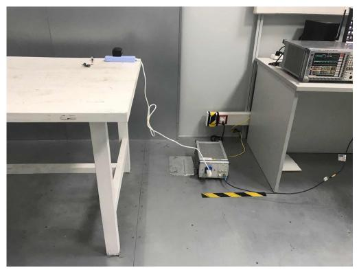
Radiated emission test 30MHz – 1GHz
