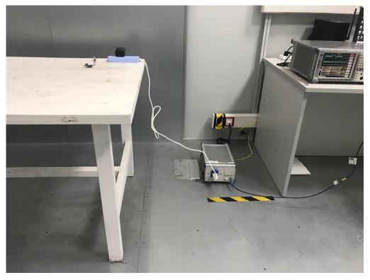
Radiated emission test 30MHz – 1GHz
