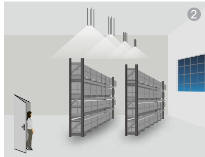
With movement and insufficient ambient lux level, the light is triggered on 100% by the detector.
