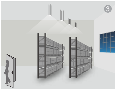
If there is no more movement, the light dims to stand-by dimming level after hold-time.
