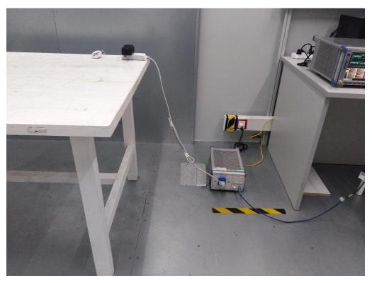
Radiated emission test 30MHz – 1GHz
