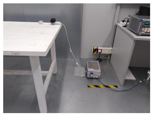
Radiated emission test 30MHz – 1GHz
