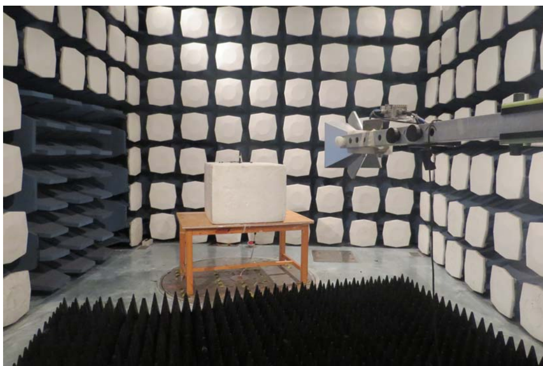
Picture 2: Radiated Spurious Emissions Test setup
