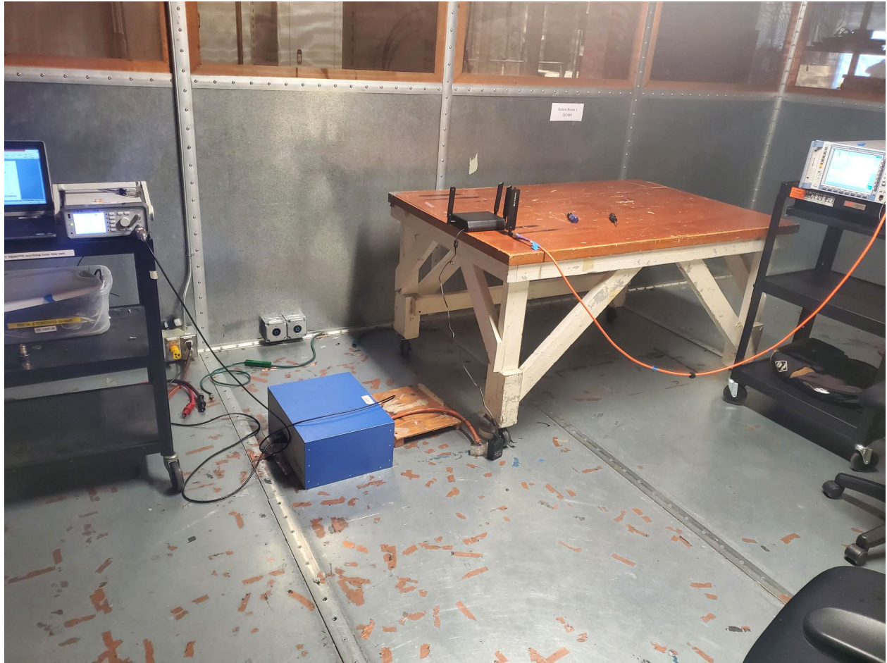
Figure 3. Conducted Emissions (AC), Test Setup
