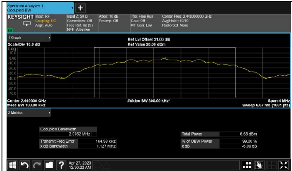
BLE-2440MHz-Data Rate- 2Mbps
