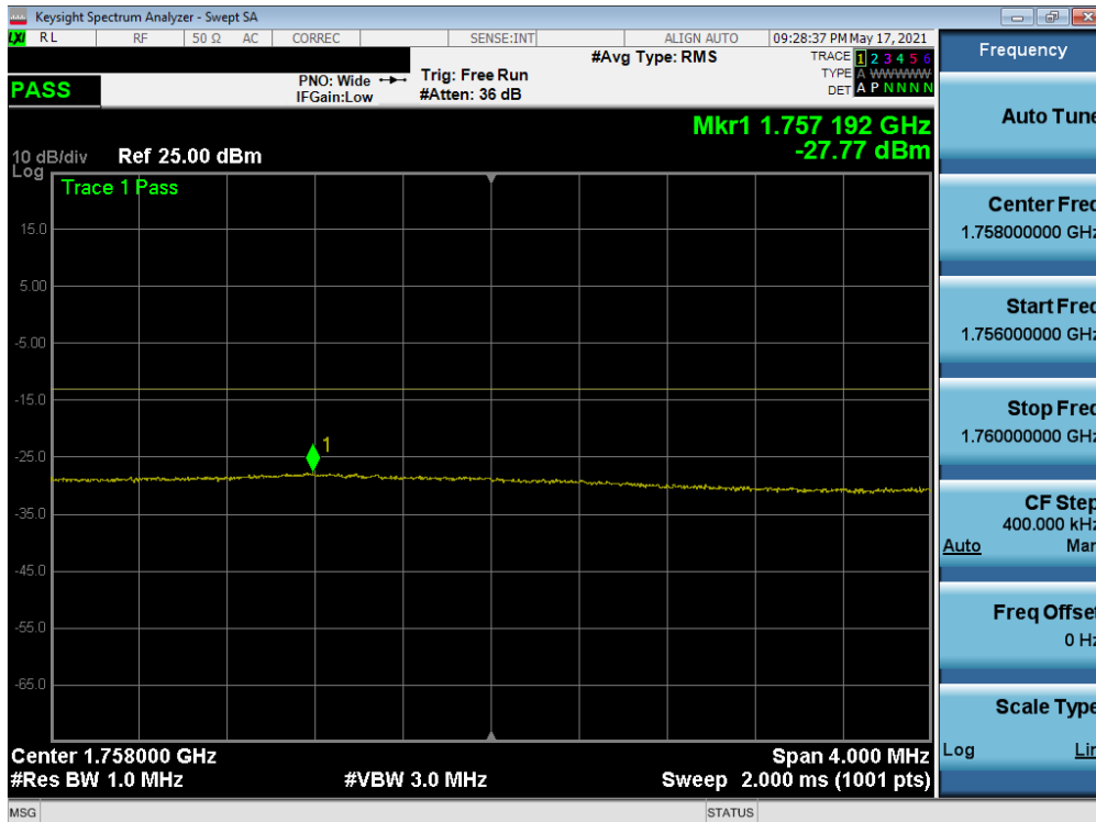
Plot 7-73. Upper Extended Band Edge Plot (LTE Band 4 - 15MHz QPSK – Full RB)
