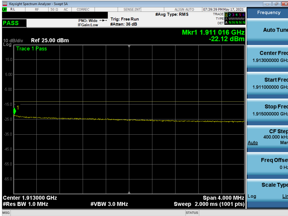
Plot 7-58. Extended Upper Band Edge Plot (LTE Band 2 - 10MHz QPSK – Full RB)
