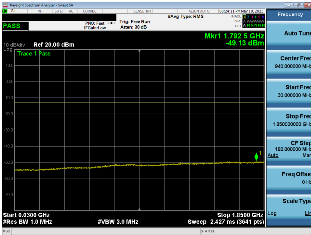
Plot 7-37. Conducted Spurious Plot (WCDMA Ch. 9400)
