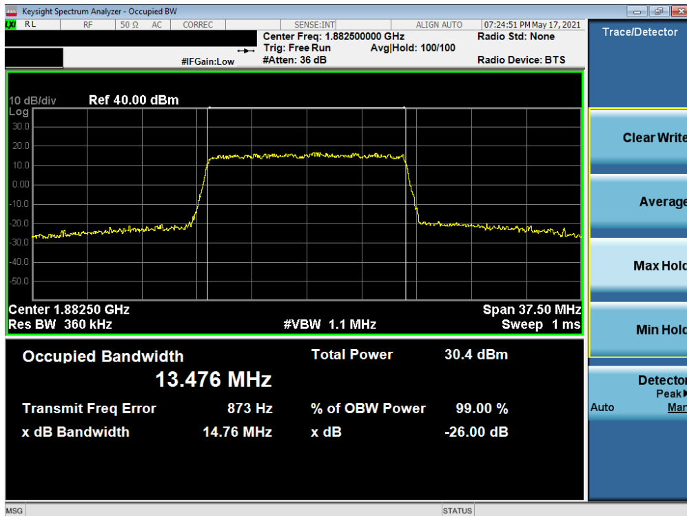
Plot 7-4. Occupied Bandwidth Plot (LTE Band 25/2 - 15MHz 16-QAM - Full RB)
