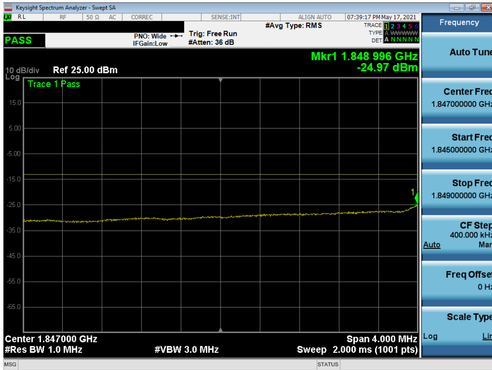
Plot 7-56. Extended Lower Band Edge Plot (LTE Band 25/2 - 10MHz QPSK – Full RB)
