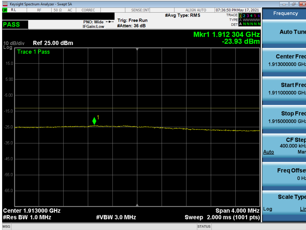
Plot 7-52. Extended Upper Band Edge Plot (LTE Band 2 - 15MHz QPSK – Full RB)
