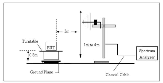
(C) Radiated Emission Test-Up Frequency Above 1GHz
