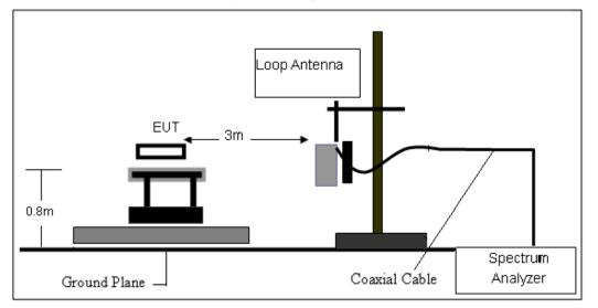
(B) Radiated Emission Test-Up Frequency 30MHz~1GHz
