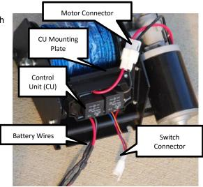
To disconnect the battery wires, first remove shrink tube. Cut with a utility knife. DO NOT cut fingers! Be careful.
